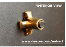
Install the bottom plate by placing the bolt into the nutsert using a 4mm allen wrench.
