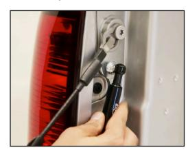
Install the narrow end of the shock on the ball mount.
